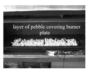
• Place a single layer of pebble on top of the burner plate.
