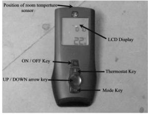
a. With the appliance lit, by pressing key the operational mode is switched from manual to Room thermostat setting and vice versa. When Room thermostat mode is active, the display shows the
